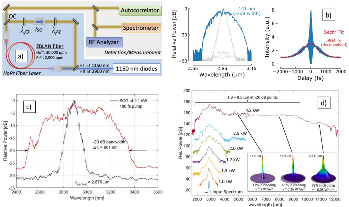
Fig. 1. (a) Schematic of the ultrafast Ho-Pr co-doped fiber ring laser. (b) Spectrally (left) and temporally (right) broadened pulse after propagation through a 8 cm long As<sub>2</sub>S<sub>3</sub> step-index fiber. (c) Spectral broadening after propagation through 39 cm of suspended core AsSe fiber. (d) Supercontinuum generated in a 5cm long As<sub>2</sub>Se<sub>3</sub> microwire. The inset shows the mode profile at various wavelengths.
