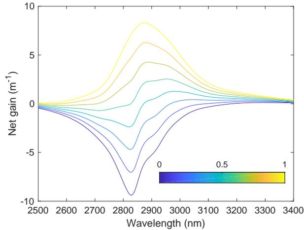
Figure 5. Net gain spectrum ( $g_{\text{net}} = \sigma_e N_2 - \sigma_a N_1$ ) as calculated from measured cross section values of  $\text{Dy}^{3+}$  in ZBLAN for increasing fractional population inversion
