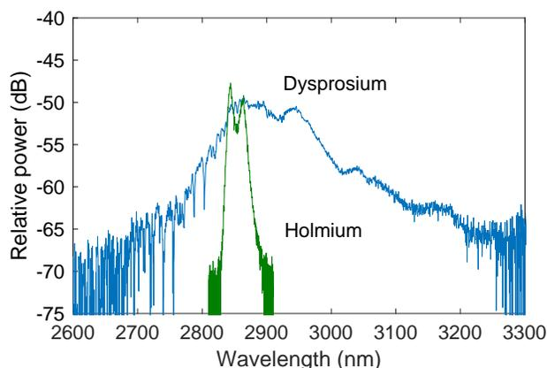
Figure 8. Measured amplified spontaneous emission (ASE) spectrum of the  $\text{Dy}^{3+}:\text{ZBLAN}$  fiber; with the measured ASE spectrum of holmium shown for comparison
