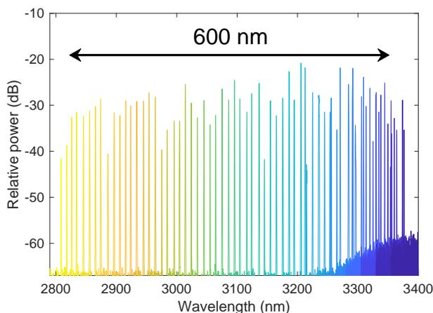
Figure 4. Measured optical spectra of laser emission over the achievable tuning range
