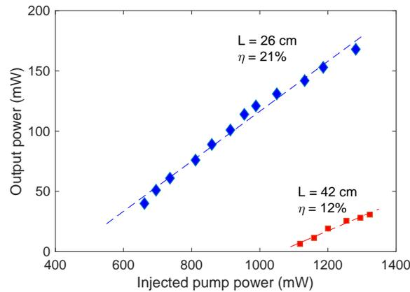
Figure 6. Laser output power as a function of injected pump power for two lengths of active fiber. A 26 cm length of fiber produces a slope efficiency ( $\eta$ ) of 21% and a maximum output power of 170 mW
