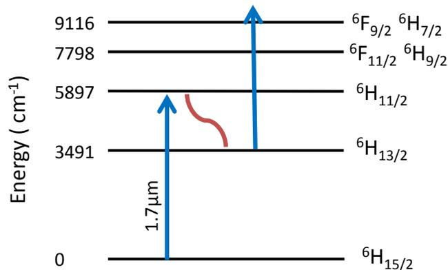
Figure 7. Energy level diagram of  $\text{Dy}^{3+}:\text{ZBLAN}$  depicting possible excited state absorption (ESA) of 1.7  $\mu\text{m}$  pump photons from the upper 3  $\mu\text{m}$  laser level (level positions from Ref. 10)
