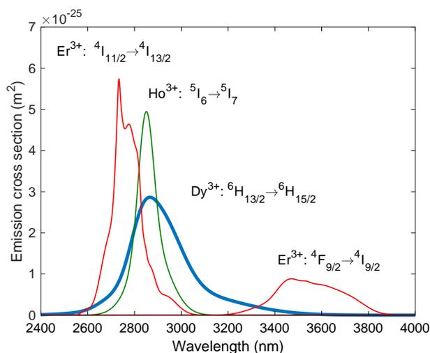
Figure 1. Emission cross sections in ZBLAN of the various mid-IR emitting rare-earth ions
