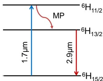
Figure 2. Simplified energy level diagram of  $\text{Dy}^{3+}:\text{ZBLAN}$  indicating pump transition, multiphonon (MP) relaxation, and 3 micron lasing transition
