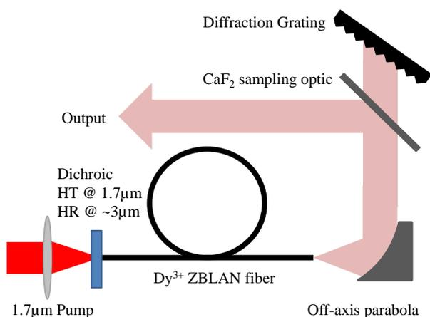
Figure 3. Laboratory schematic diagram of the tunable dysprosium fiber laser
