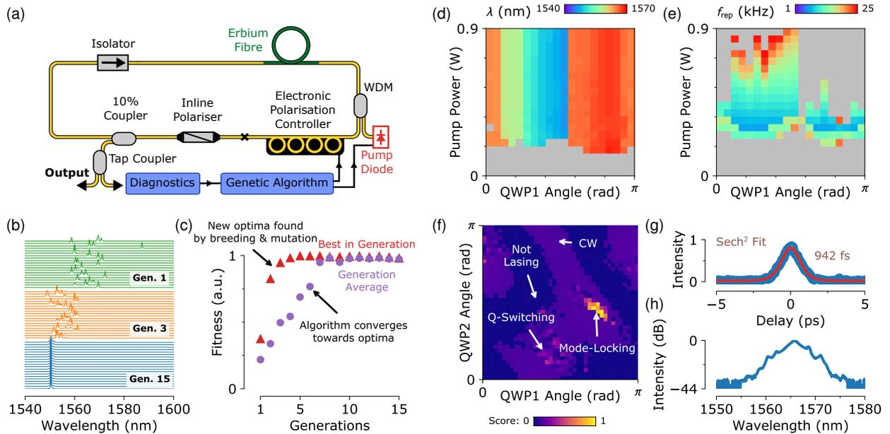
Fig. 1. (a) Cavity schematic; (b)–(c) Self-tuning spectral evolution; (d) wavelength and (e) Q-switched repetition rate variation with 2 parameters varying (other 3 fixed); (f) variation of fitness in 2D parameter space, showing small mode-locking regime; (g) autocorrelation and (h) spectrum.
