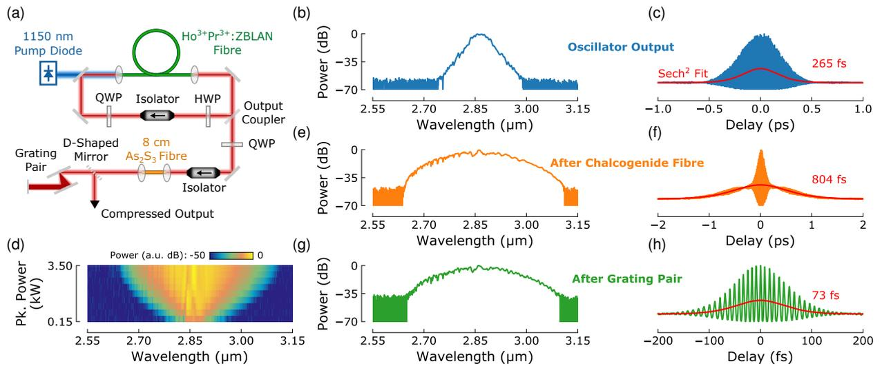
Fig. 1. (a) Experimental setup; (b-c) Ho:ZBLAN oscillator output pulse spectrum and autocorrelation trace; (d) Spectral broadening in  $\text{As}_2\text{S}_3$  fibre as a function of launched peak power; SPM-broadened (e-f) and compressed (g-h) pulse spectrum and autocorrelation trace.
