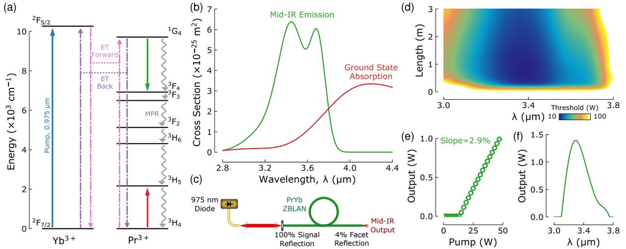
Fig. 1. (a) PrYb energy levels; (b) mid-IR cross sections; (c) cavity design; modelling results: (d) pump threshold variation with signal wavelength and fibre length; (e) 3.4  $\mu\text{m}$  output power against pump for 0.5 m length; (f) variation of output power with wavelength for 50 W incident pump.
