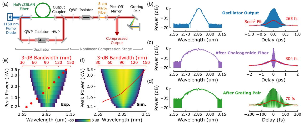
Fig. 1. (a) Experimental setup; (b) Ho:ZBLAN oscillator output pulse spectrum and autocorrelation trace; SPM-broadened (c) and compressed (d) pulse spectrum and autocorrelation trace; spectral broadening in  $\text{As}_2\text{S}_3$  fiber as a function of launched peak power, (e) experimental and (f) numerical.
