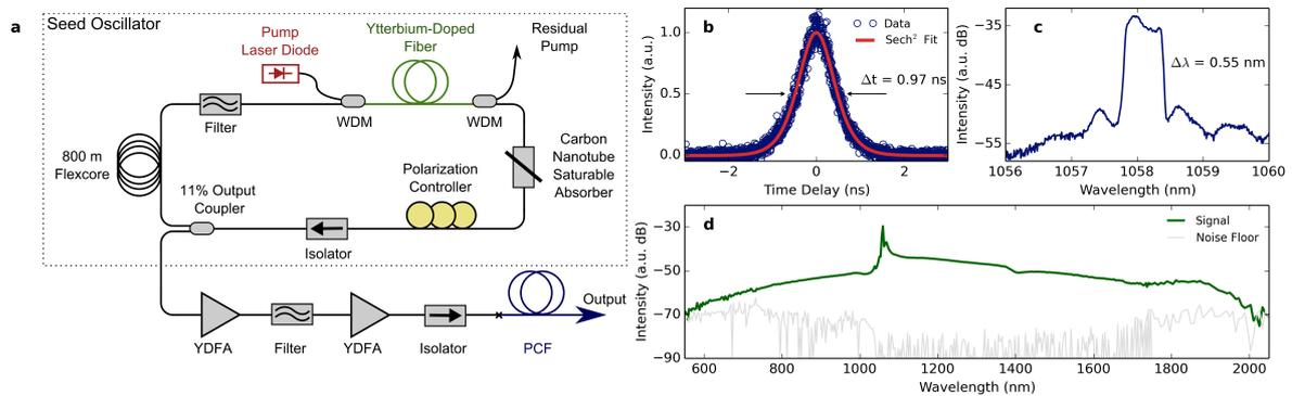
Fig. 1. (a) Laser setup. Seed oscillator pulse (b) temporal profile and (c) spectrum. (d) Supercontinuum after PCF.
