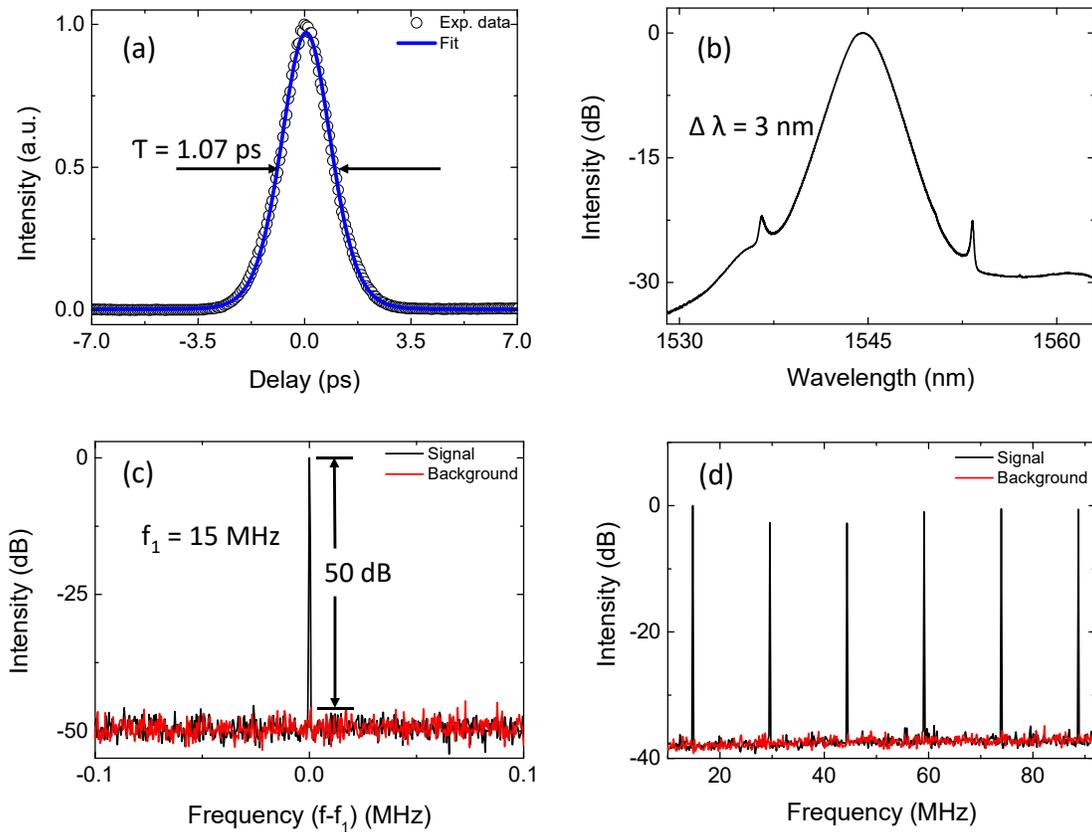
Fig. 2. (a) Measured optical spectrum. (b) The corresponding experimentally measured intensity autocorrelation. (c) Fundamental radio frequency on a span of 200 kHz, where  $f_1=15$  MHz is the fundamental cavity frequency. (d) Harmonic radio frequency spectrum on a span of 80 MHz.
