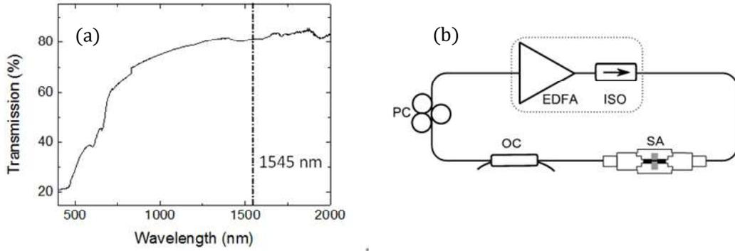
Fig. 1. (a) Linear transmission of MoS<sub>2</sub> saturable absorber. The dashed line indicates the wavelength of operation. (b) Schematic of the Er-doped fiber laser cavity: EDFA: erbium-doped fiber amplifier; ISO: isolator; SA: saturable absorber; OC: fiber output coupler; PC: polarization controller.
