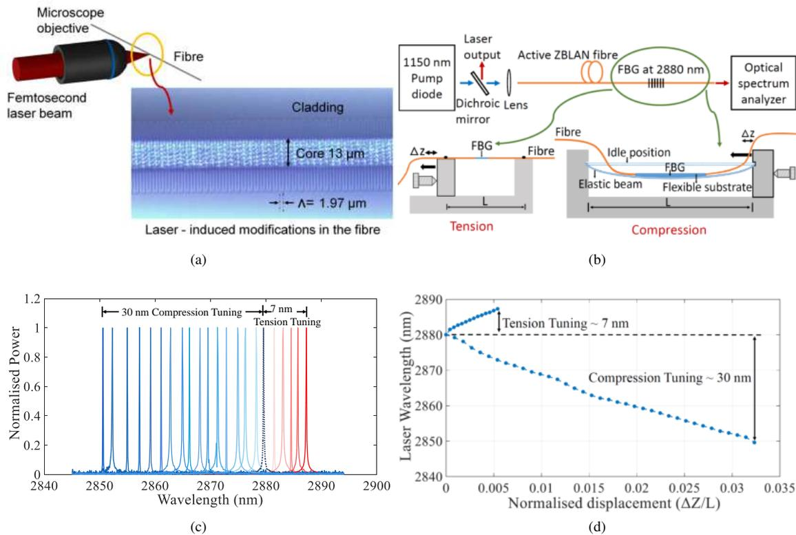
Figure 1. (a) Femtosecond laser direct-write setup and microscopic image of the FBG (b) Experimental setup (c) Spectra of the shifted laser output peaks. Note that the laser linewidth across the entire tuning range was less than 112 pm (d) Measured tuning range of the tunable laser source
