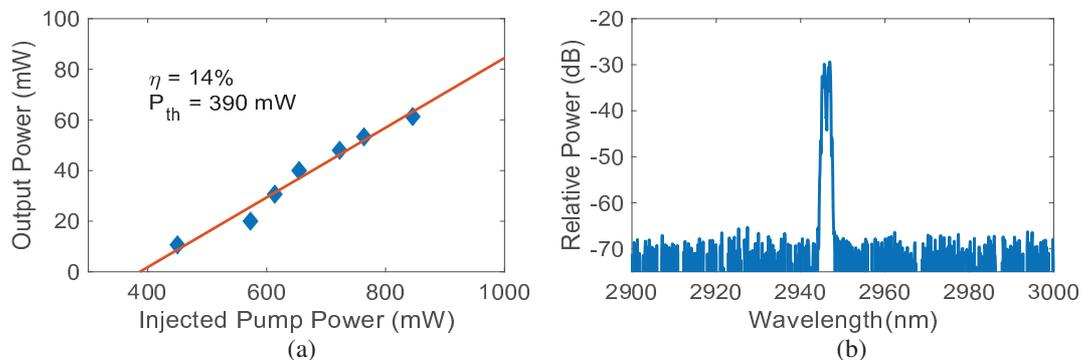
Fig. 3. (a) 3  $\mu\text{m}$  output power as a function of injected pump power; slope efficiency ( $\eta$ ) is 14% with an oscillation threshold of 390 mW (b) Measured optical spectrum of the 3  $\mu\text{m}$  output; emission is centered around 2945 nm.
