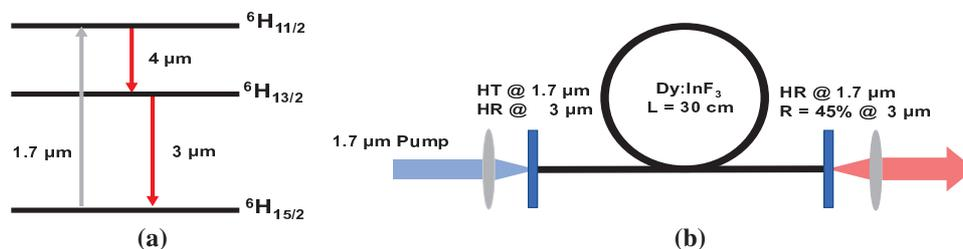
Fig. 1. (a) Simplified energy level diagram of dysprosium showing ground state pump absorption and both mid-IR radiative transitions. (b) Experimental schematic; indicated dichroic cavity mirrors are removed for 4  $\mu\text{m}$  emission measurement.
