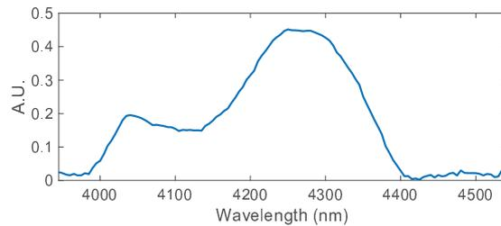
Fig. 2. Monochromator measurement of emission beyond 4  $\mu\text{m}$  from the  $\text{Dy}^{3+}:\text{InF}_3$  fiber
