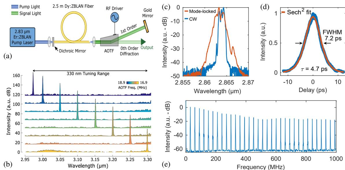
**Fig. 1** a) dysprosium FSF cavity; b) tuning range of pulsed output for the Dy system; holmium-doped system performance; c) optical spectrum exhibiting broadening; d) autocorrelation trace with deconvolved pulse width of 4.7 ps; e) RF photodiode signal with multiple harmonics of the cavity round trip time.
