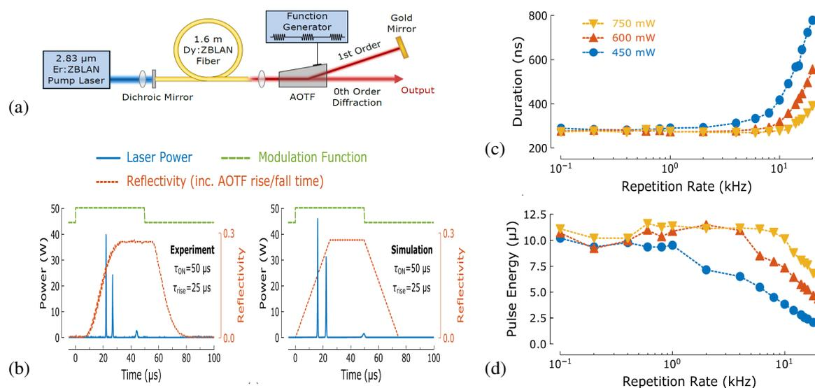
**Fig. 1** a) laser schematic; b) comparison of numerical simulation to experiment identifying multiple pulse regimes; c) pulse duration as a function of repetition rate; d) pulse energy as a function of repetition rate.
