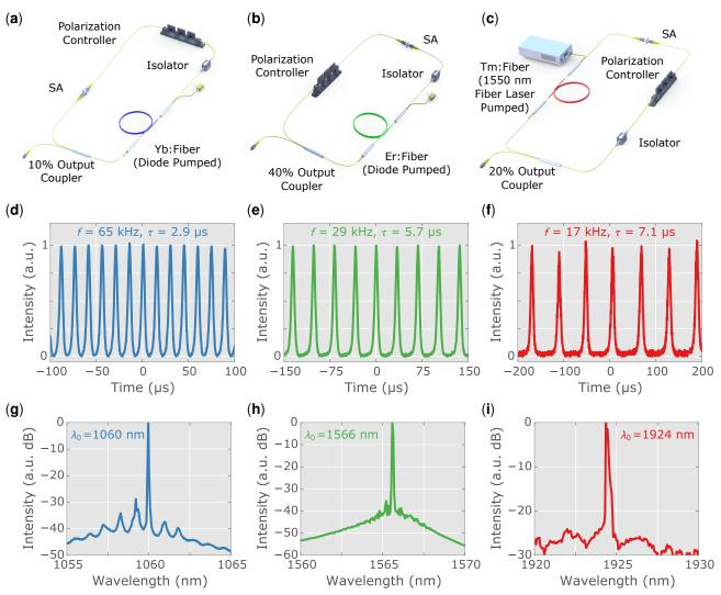
**Figure 5.** Q-switched fibre lasers with MoSe<sub>2</sub>-PVA saturable absorber, after [55]: (**a**–**c**) cavity schematics; (**d**–**f**) output pulse trains showing the repetition rate f and pulse duration  $\tau$ ; (**g**–**i**) spectra. The columns (left to right) show Yb, Er and Tm laser results.
