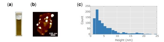
**Figure 3.** Fabrication of few-layer  $MoS_2$  flakes by liquid-phase exfoliation (LPE), after [32]: (a) liquid dispersion of flakes; (b) AFM image; (c) distribution of flake heights from AFM.
