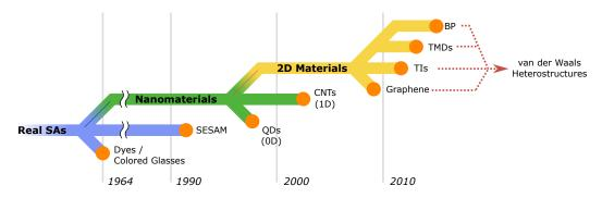
**Figure 1.** The evolution of real saturable absorber technologies. Orange dots denote the first reported application of each technology in a pulsed laser.
