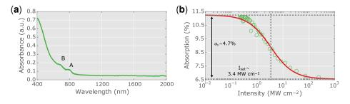
**Figure 4.** Characterization of  $MoSe_2$ -PVAcomposite, after [55]: (a) linear absorption; (b) Z-scan measurement, fitted with a two-level saturable absorber (SA) model (solid red line) to determine device performance parameters. Labels A and B refer to excitonic transitions, as described in Section 2.1.
