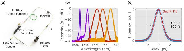
**Figure 6.** Tunable mode-locked Er:fibre laser using  $MoS_2$ -PVA saturable absorber, after [37]: (a) cavity schematic; (b) examples of optical spectra from the continuous tuning range of 1535–1565 nm; (c) autocorrelation trace at 1552 nm (assuming sech<sup>2</sup>-shaped pulses, the deconvolution factor is 1.55).
