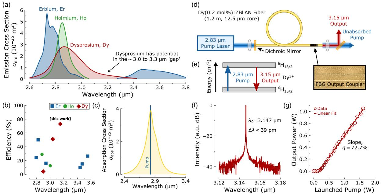
Fig. 1. (a) Emission cross sections for Er-, Ho- and Dy-doped ZBLAN; (b) maximum slope efficiencies for mid-IR fiber lasers to date (adapted from Ref. [9]); (c) Dy:ZBLAN absorption cross section; (d) cavity schematic; (e) Dy energy level diagram; (f) laser spectrum; (g) laser power characteristic.
