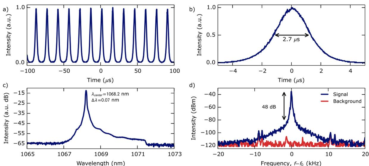
Fig. 2. Q-switched laser characteristics: (a) pulse train; (b) pulse profile; (c) optical spectrum; (d) RF spectrum,  $f_0=67$  kHz.
