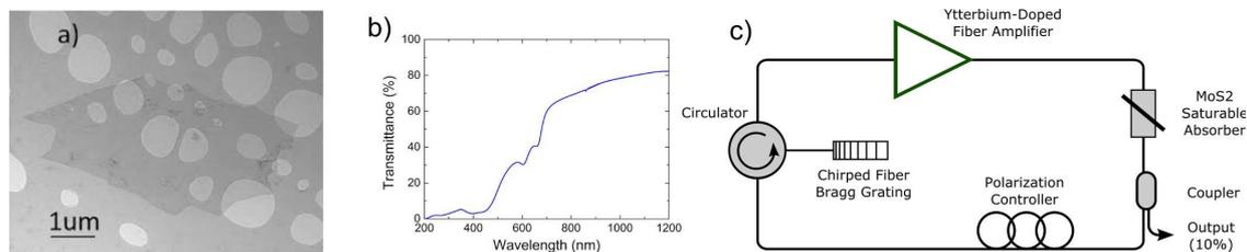
Fig. 1. (a) TEM image of an MoS<sub>2</sub> flake; (b) Transmission spectrum of MoS<sub>2</sub>-polymer composite; (c) Laser cavity schematic.
