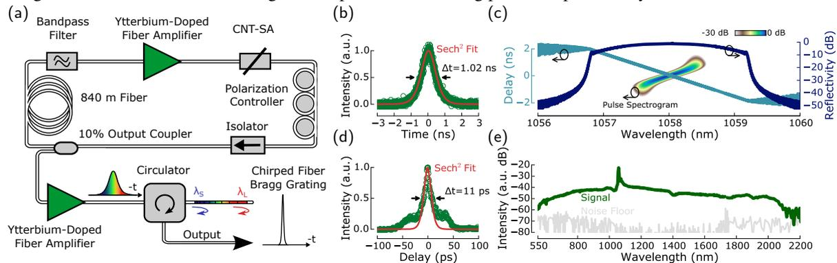
**Fig. 1** (a) System setup. (b) Pulse profile from ultra-long laser. (c) Simulation results: pulse spectrogram overlaid with CFBG reflectivity and CFBG group delay. (d) Compressed pulse autocorrelation trace. (e) Supercontinuum after PCF.
