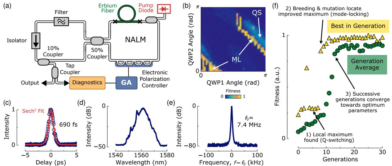
Fig. 1. (a) Cavity schematic. (b) Map of fitness values in a subset of parameter space. (c) Autocorrelation, (d) optical spectrum and (e) RF spectrum in a stable fundamental mode-locking regime. (f) Evolution of fitness score, demonstrating convergence of successive generation's average value towards the maximum, using our genetic algorithm. NALM: nonlinear amplifying loop mirror.
